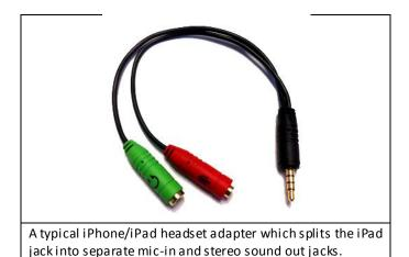
In order to use an independent (external) microphone with the iPad, it is necessary either to use a device with a jack specifically designed to connect only to pins 3 and 4, or in conjunction with an adapter which will separate these pins for the mic and sound out functionality as shown above.
